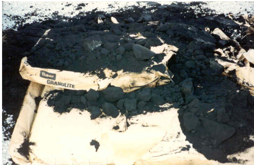
Figure 14 Ground Tire Rubber Used in Asphalt Rubber Binder
